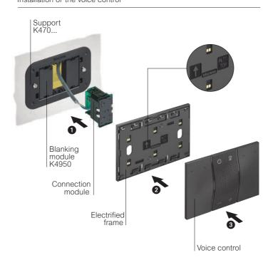
Remove the finishing bars from the electrified frame. When installing power supply item K8003, connection module item K8001 must not be used.
