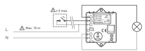
Option: remote control through mechanical pushbutton, not luminous.
