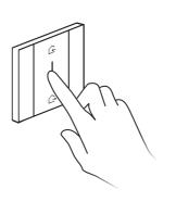
**B.** Place the devices to be associated in contact
