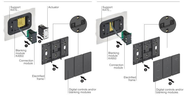
Use in conjunction with the connection module, or another actuator, to take up the power voltage.
