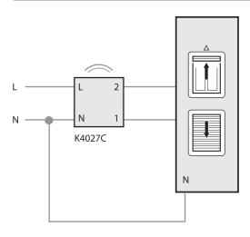
Warning: only compatible with standard motors (no pulse motors, no radio motors)
